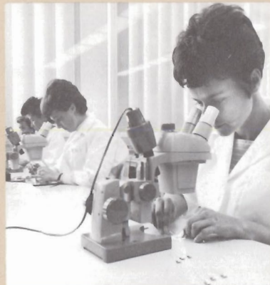
Assembling tiny tape-head parts under microscope are, from right: Jacqueline Vuille, Priscilla Bumbaca, Yuri Kafai, Dee Carver.
