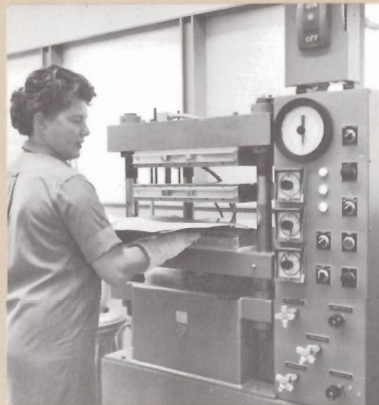
Marybeth Carpenter takes laminated printed circuits from hot press where four, six, and eight layers are fused into one board.
