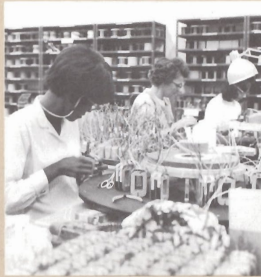
Paeco transformers pass through many steps of production. From left, Bettye Allen, Joan McDonald, and Rosie Steele hook up headers.
